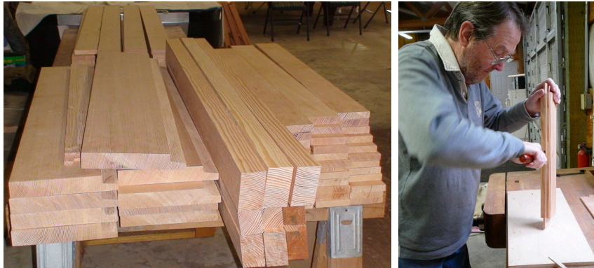
Freshly milled materials, Derek Tetlow cleaning out a mortise for glass panel.
